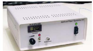
Laser activation is controlled with the ON and OFF switch on the front panel and the power level is adjusted by the potentiometer on the front panel. The turn-on and turn-off response time of the driver circuit is approximately 2 msec, allowing modulation of the laser output at a maximum frequency of approximately 200 Hz.
