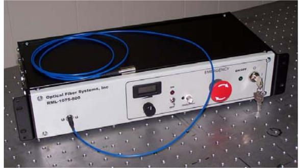
Laser activation is controlled with the ON and OFF switch on the front panel and the power level is adjusted by the potentiometer on the front panel. The turn-on and turn-off response time of the driver circuit is approximately 2 msec, allowing modulation of the laser output at a maximum frequency of approximately 200 Hz.
